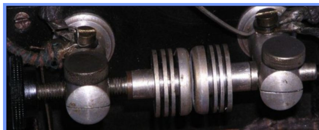
Figure 2. Spark unit of Army transmitter (Kurrajong Radio Museum)
