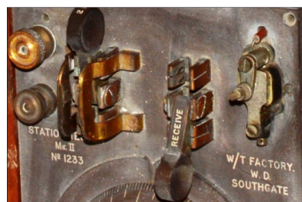
Figure 2. Spark unit of Army transmitter (Kurrajong Radio Museum)
